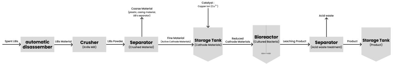
Fig. 3. Process Flow Diagram of Pilot Scale Bioleaching from Spent Lithium-Ion Batteries.
